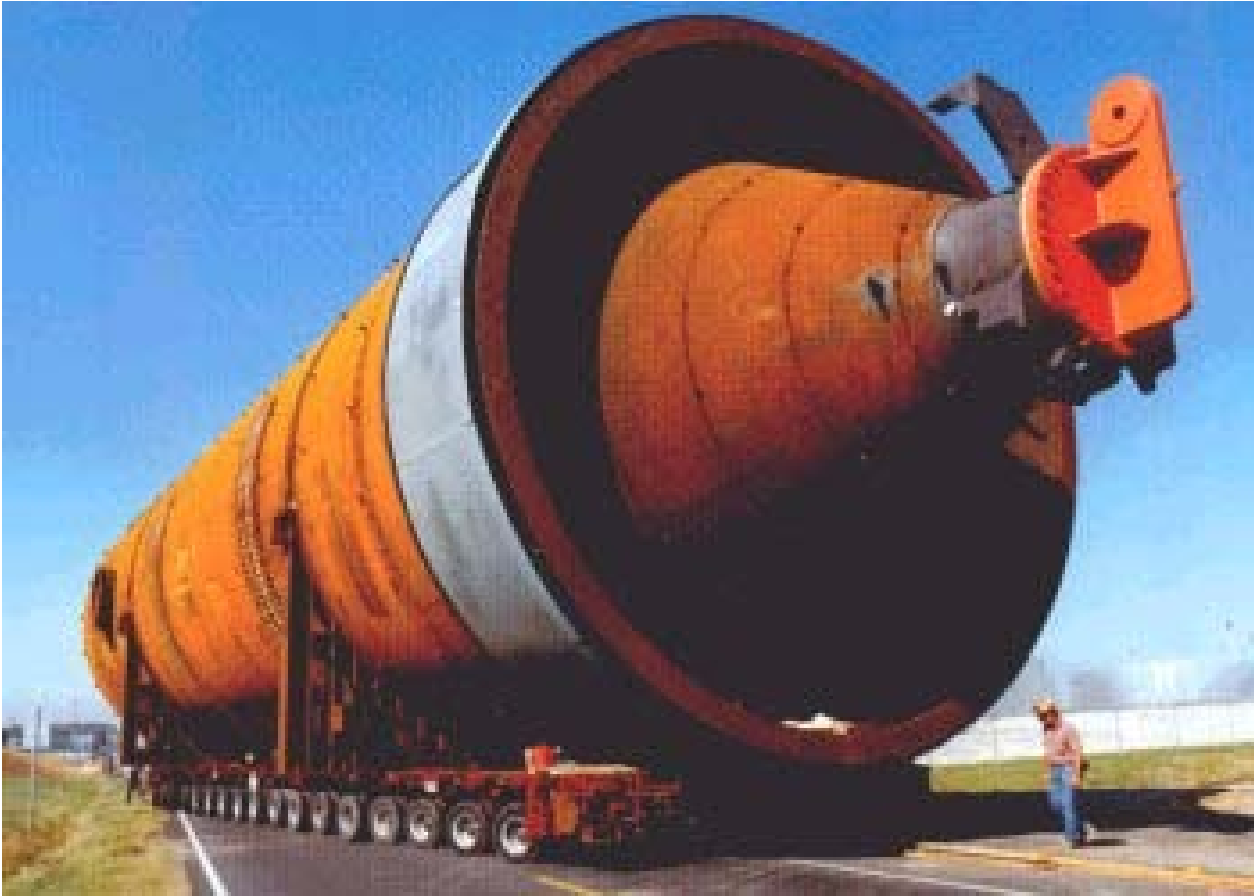
Transporting 550 ton Coker Drum from ship to crane hook
